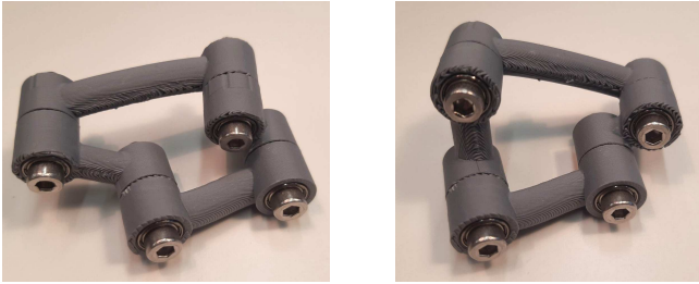
Fig. 4: Physical model of a snapping four-bar, produced by D. Huczala
