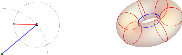
Fig. 2: (left) 2-R planar mechanism. The blue arm revolves about the fixed point, while the red arm is connected with a revolute joint to the second endpoint of the blue arm. (right) The configuration space of the 2-R planar mechanism. The blue and red circles represent the respective rotations of the arms.
