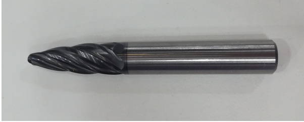
Fig. 1: A curved tool for 5-axis flank CNC machining.
