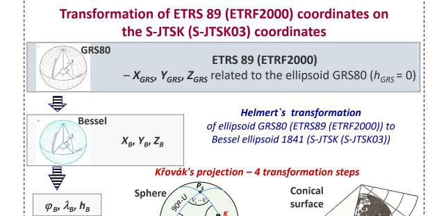
Conical conformal projection in the oblique position, scale distortion ±11.8 cm/km
